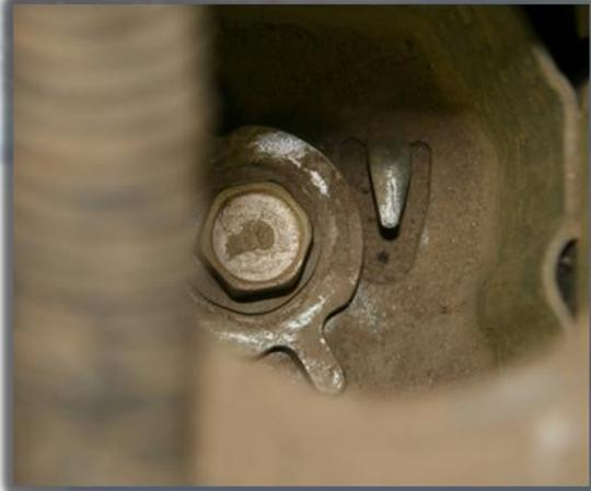
15. If using an auto shop lift. Lift both sides of the body. If using a floor jack only lift one side of the body at a time. Only lift the body high enough so that the spacers can slide between the body and the bushings on the frame. **NOTE THE BODY SHOULD LIFT EASILY. IF THE BODY HAS ANY HESITATION STOP AND FIND WHAT IS STOPPING THE BODY FROM COMING OFF THE FRAME.**
