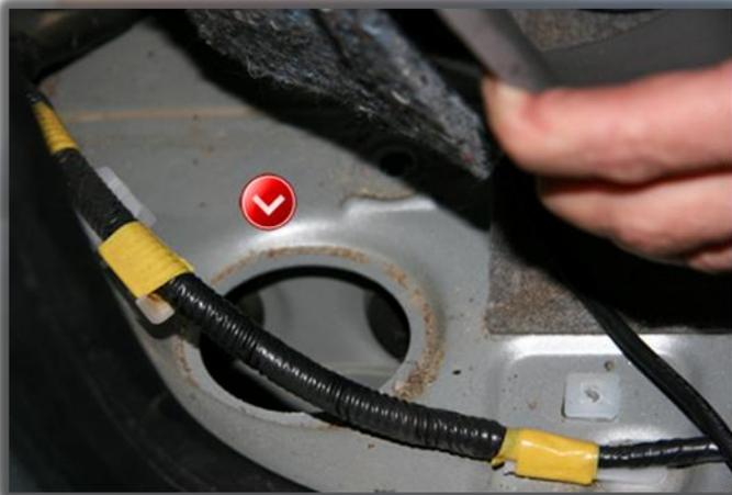
10. The body mounts in the middle, take off the plastic trim on the sides of the rear seats. Lift up the carpet and you will see the hole that leads to the body mount in front of the rear tire.
