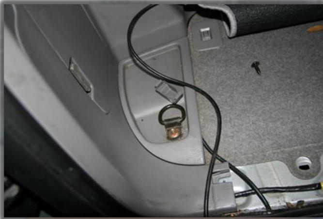
9. Pull the side panels away and expose the holes that lead you to the rear body mounts.
