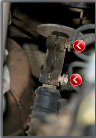
5. Drop the spare tire to allow access to a centering bracket on the body. Bend the centering bracket up to allow for reinstallation of the spare once the lift is complete.
