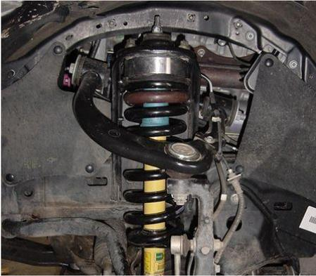
18. Reinstall the lower ball joint bolts and sway bar. **If your kit came with a front diff drop kit, now is a good time to install it.** Reinstall the wheels/tires and skid plate. Torque all nuts and bolts to manufacturer specs.
