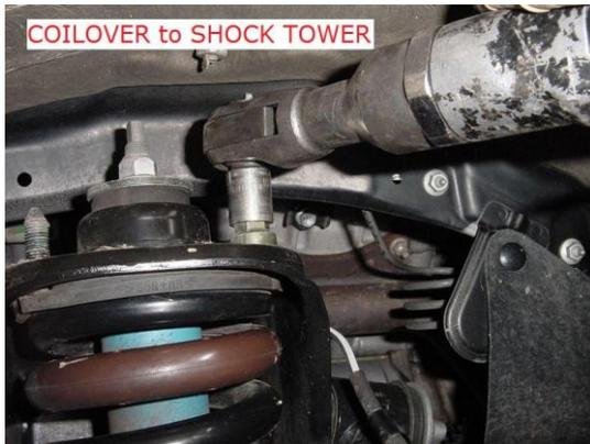
10. **Being careful not to overextend and pull apart the inner CV Axle joint**, move the spindle/hub assembly out of the way so the coil-over can be removed from the vehicle. Remove the coilover on both sides.
