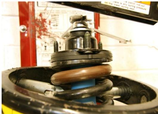
14. **3" LIFT KITS ONLY**- Remove the three top plate studs on each of the top plates. This can be accomplished with a vice and large deep socket, or by placing a large deep socket on the concrete and hammering them out. Replace O.E. studs with new longer bolts supplied in your kit.
