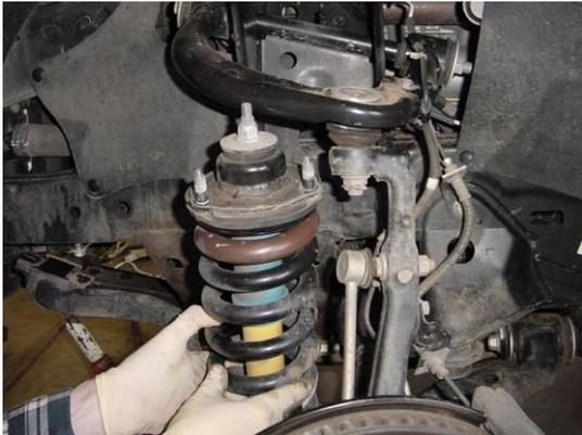
11. **Before compressing the coils, note the alignment of the top plate stud in relation to the lower shock eyelet hole. The stud which is closest to the engine is aligned directly down the center of the strut body, 90 degrees from the bottom shock eyelet hole center.**
