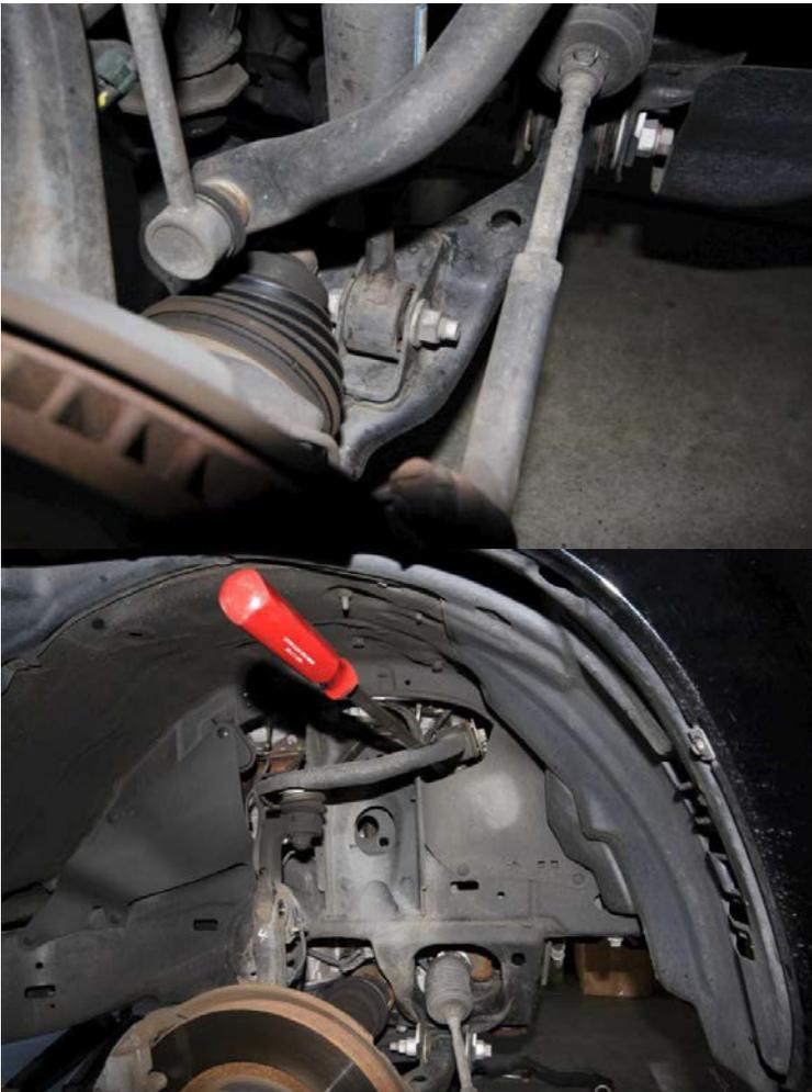
8. Remove the 3 top bolts holding the strut assembly to the frame.
