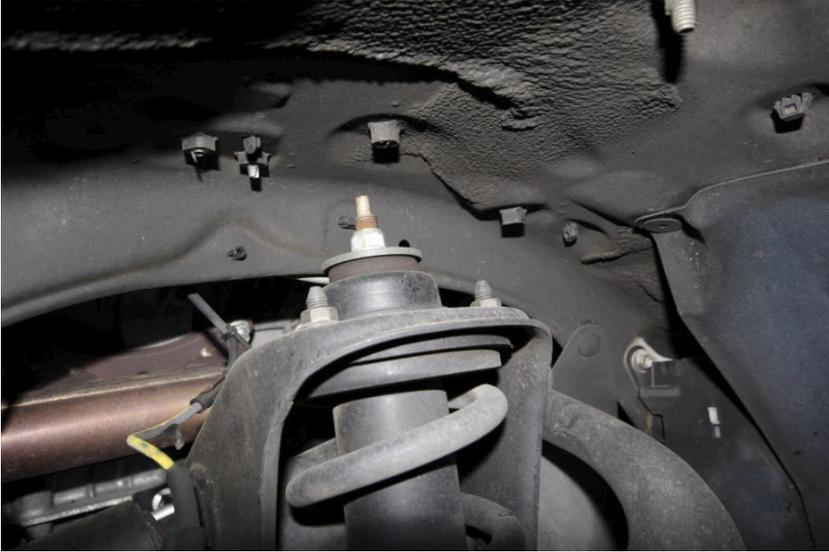
9. Push down on the upper control arm with a pry bar while moving the strut out of the lower mount and down slightly. Then slide it out towards the front while releasing the pry bar and moving it out underneath the upper control arm.
