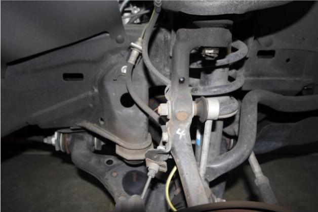
4. Now undo the bolts holding the swaybar bushing brackets and then remove the swaybar from the vehicle. **Tip:-** The front 2 holes on the bracket are open allowing you to slide the bracket out. Thus remove the 2 bolts to the rear and then undo the 2 front, but don't remove. Then simply slide the bracket and swaybar out towards the rear.
