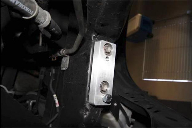
16. Install the swaybar and swaybar brackets on the spacers. Make sure that the swaybar ends push in above the CV axles on each side. Note the tip in step 4 and apply in reverse. Torque the swaybar spacer bolts to **30ft/lb.**
