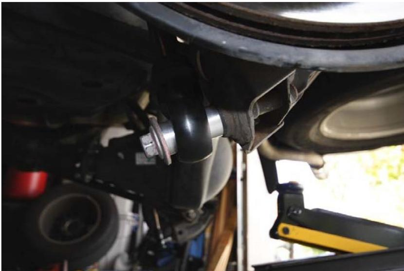
7. Tighten the top shock absorber mount nuts. . Please note the following when installing your ToyTec shocks product with a pin mount on the end cap (generally the top of the shock):
