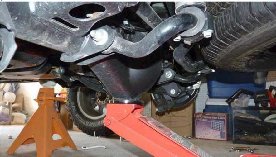
3. Undo and remove the lower shock absorberbolts.
