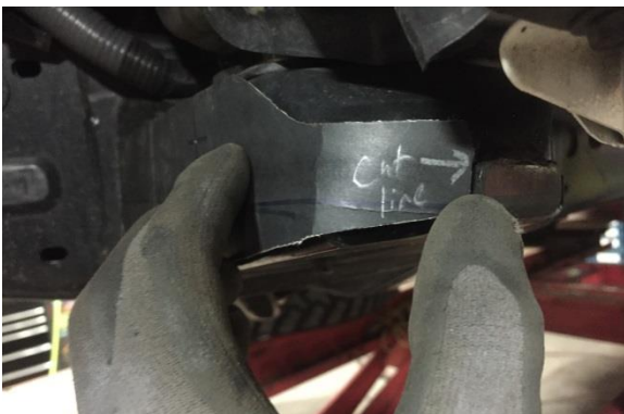
2: Cut out template and place along front facing edge of the body mount. Transfer end and center marks onto the frame.
