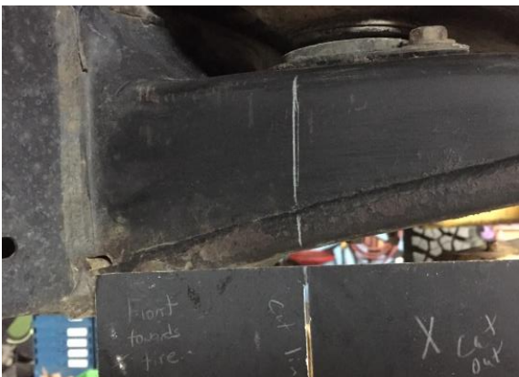
3: After transferring your marks onto frame, draw a straight line along the bottom surface of mount from the center mark to edge mark. This will allow the body mount chop filler plate to angle away from your tire.
