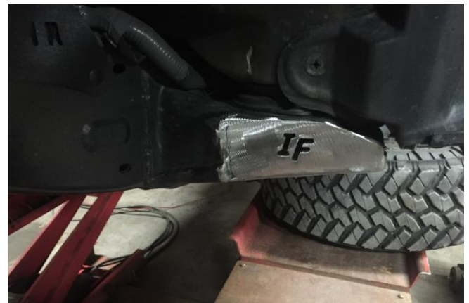
5: Tack filler plate onto frame. Make sure it is angled away from tire at the bottom. If there are any lips jutting into wheel well grind them down to match filler plate.
