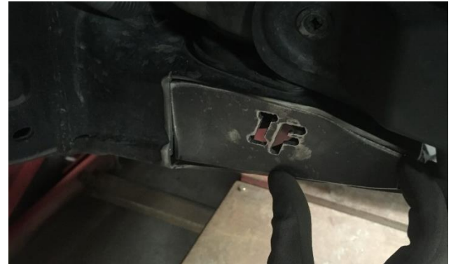
4: Using filler plate as a guide remove material back to your lower mark line, leaving upper frame material at the corner as to not disturb factory body mount.
