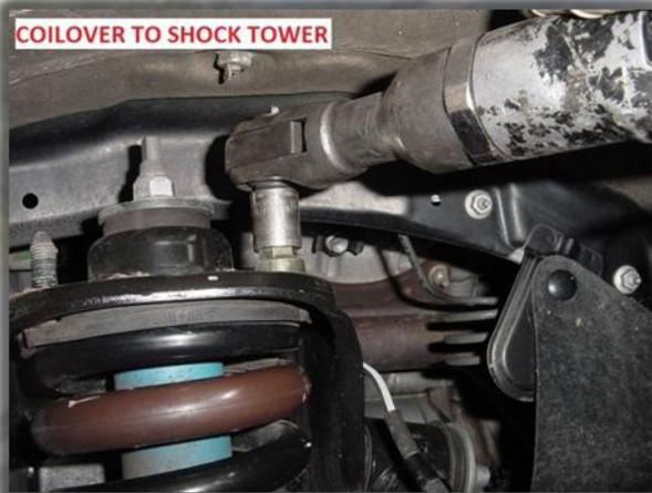
10. Being careful not to overextend and pull apart the inner CV Axle joint, move the spindle/hub assembly out of the way so that the coilover can be removed from the vehicle. Remove the coilover on both sides.
