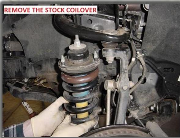
11. Before compressing the coil, make note of the stud orientation in relation to the lower shock eyelet hole. The stud which is closest to the engine is aligned directly down the center of the strut body, 90 degrees from the center bottom shock eyelet hole.
