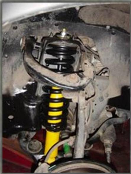
20. Reinstall the lower ball joint bolts, sway bar, wheels/ tires, and the skid plate. Torque all of the bolts and nuts to manufacturer specs.
