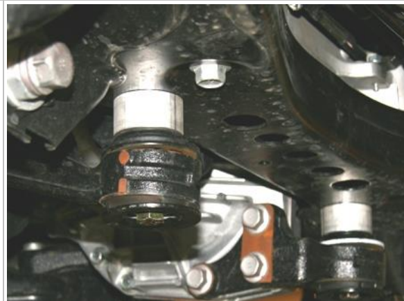
Diff Drop kit Installed (Fig. 2)
