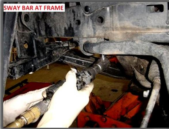
7. Remove the lower shock nut and bolt.
