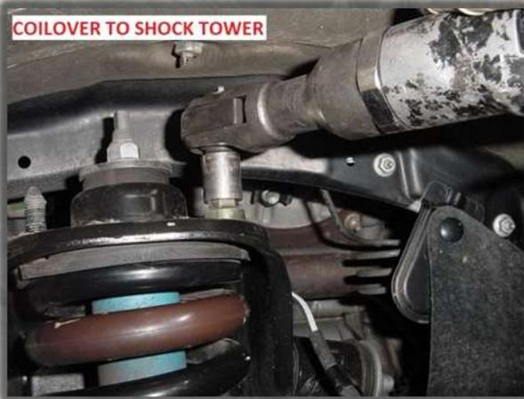
10. **Being careful not to overextend and pull apart the inner CV Axle joint,** move the spindle/hub assembly out of the way so that the coilover can be removed from the vehicle. Remove the coilover on both sides.
