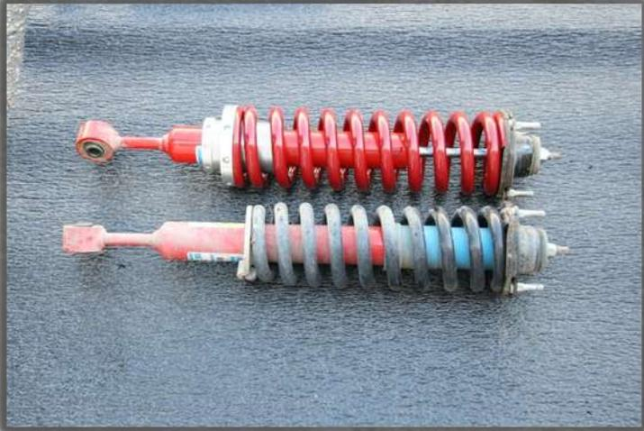
20. Position the coilover onto the vehicle, sliding the top into the shock tower first. Install the top three nuts which hold the coilover to the shock tower and tighten finger tight. Install the lower shock bolt and nut. You may need to pry down on the upper control arm in order to get the lower shock bolt installed. Torque upper nuts and lower bolt/nut to manufacture specs.
