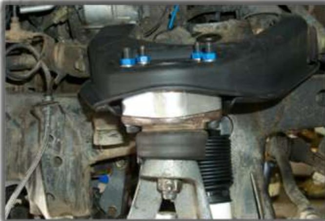
11. Tighten ball joint hardware to 30 ft. lbs. or 40 N.m. **NOTE: Apply this torque to the allen head bolt and the Grade 10.9 nut only, then install the 2nd nylon lock nut and tighten it down snugly in order to lock the first nut in place. No need to toque the nylon lock nut to 30 ft. lbs. as well, it may strip.**
