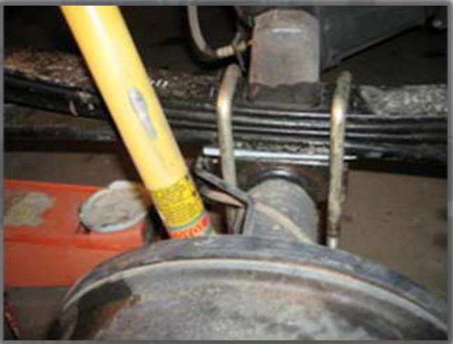
14. Re-install all bump stops, U-bolts, axle plates, washers, and nuts. Torque U-bolt nuts to manufacturer specs.
