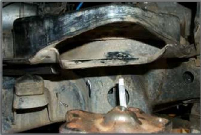
6. Knock the studs out of the ball joint with a small hammer. This is done most easily if the joint is pressed against the arm supported with a floor jack
