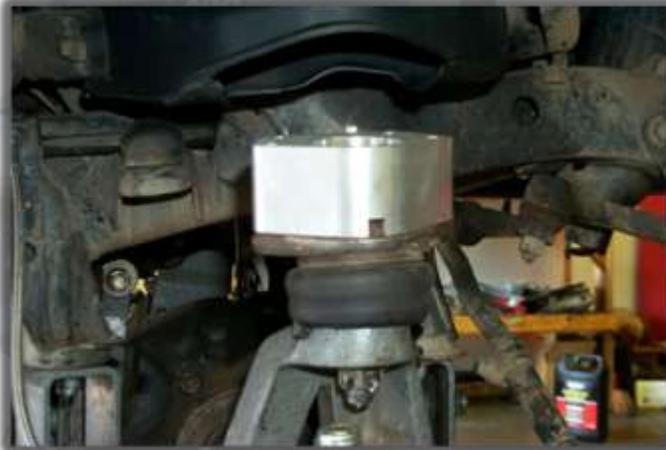
10. Using a floor jack to control arm height, align the ball joint and install the hardware.
