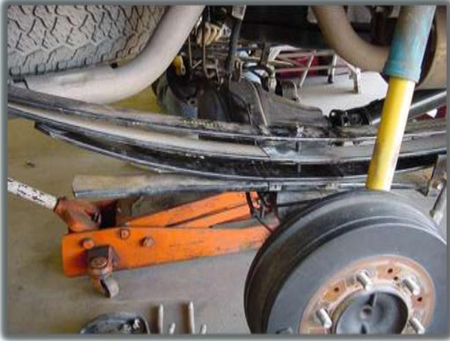
13. Jack the axle back into place and ensure the center bolt head on the spring pack sets into the hole on the axle spring perch. **If your lift kit is supplied with axle shims, place the center bolt head through the shim center hole and into the spring perch. The thinner end of the shim should face toward the front of the vehicle.**
