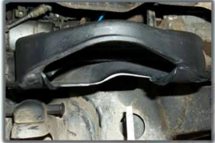
9. Put the spacer in place, NOTCH FACING DOWNWARD. The notch acts as a weep hole to let any water that gets in from above drain out to prevent the ball joint from rusting out.
