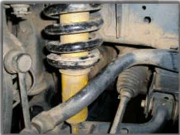
15. Secure and compress the new spring. Install the new shock, washers, bushings, spring isolator, top plate, remaining washers, bushings and top nut in the reverse order as disassembly. Double check that the top plate bolts is aligned correctly with the bottom of the shock, before and while uncompressing the coil. Repeat assembly for the other side. Make sure to remember which side is the driver side.
