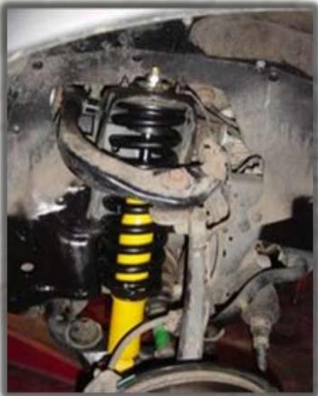
18. Reinstall the lower ball joint bolts, wheels/ tires, and the skid plate. Torque all of the bolts and nuts to manufacturer specs.
