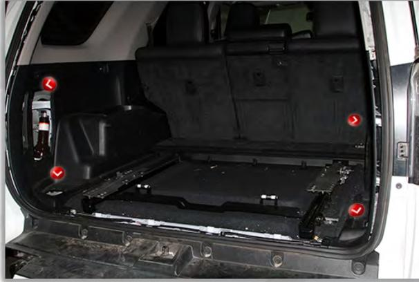
Pull the side panels away in the cargo area and expose the holes that lead you to the rear body mounts.
